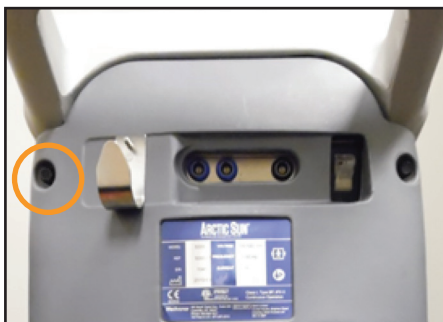
Fig. 8-72 Ta bort bult (steg 1)
