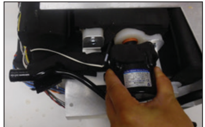
Fig. 8-47 Monter pumpen igen (trin 6) (to visninger)
